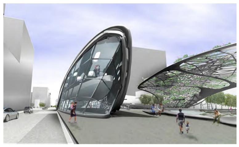
solar collectors provide energy, collected rainwater provides water for the green park and greenhouses and also expresses itself in fountains providing cooling through 'misting'.
