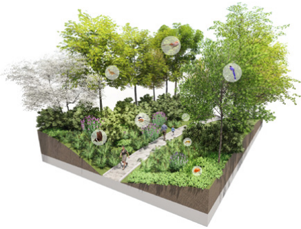
Figure 8.9 Archi-Tectonics, Asian Games, Hangzhou, China, 2022: Perspective showing the varied topography of the Asian Games Park supporting storm water absorption. Much of the planted earth was first bermed as part of a zero-earth strategy to redeposit soil mass within the site boundaries. The result was a gradually sloped synthetic nature – a hybrid landform/building that created diverse view corridors while passively channeling light and air within the constructed section of the site.
