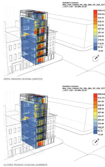
Figure 8.2 Archi-Tectonics, Greenwich Street Building, New York, NY, 2000. Folded double glazing with a solar film allows the glass façade to perform specifically for the New York climate. The glazing allows for solar penetration from the low winter sun, providing passive solar energy, while the solar film protects from the harsher summer sun, removing solar glare. Such an example of form-as-performance, articulated by Manuel DeLanda and others, was an early goal of architects engaging the digital.
